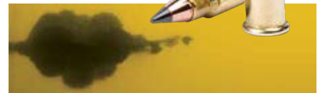
A17 17 HMR (949CC) shot into bare ballistics gel at 100 yards; 6 inches penetration.
